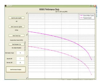
Figure 5(c): AES+Huffman under AWGN channel
