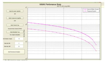
Figure 5(a): AES+DWT under AWGN channel
