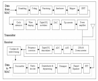
Figure 1: OFDM transceiver block diagram
